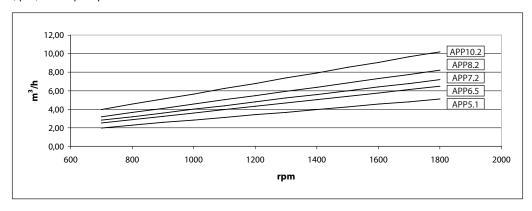
Furthermore, this diagram shows that the flow can be changed by changing the rotation speed of the pump. The flow/rpm ratio is constant, and the "desired" flow can be obtained by changing the rotation speed to a corresponding value. Thus, the required rpm can be determined as:
