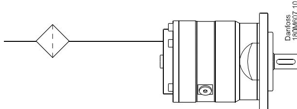
In order to avoid the risk of cavitation, the inlet pressure at the pump must be min. 0.9 bar (13 psi) abs.
