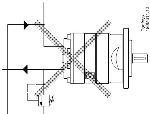
The valve should be placed as close to the pump as possible.
