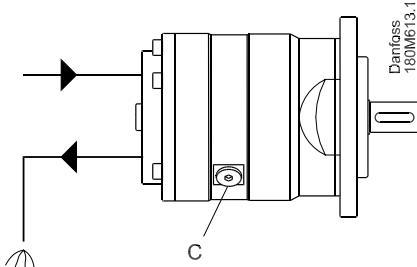
At the initial start of the system, the pump should be run without pressure for about 5 minutes, thus removing possible impurities from pipes, hoses, etc. However, the system should be flushed before start-up.
