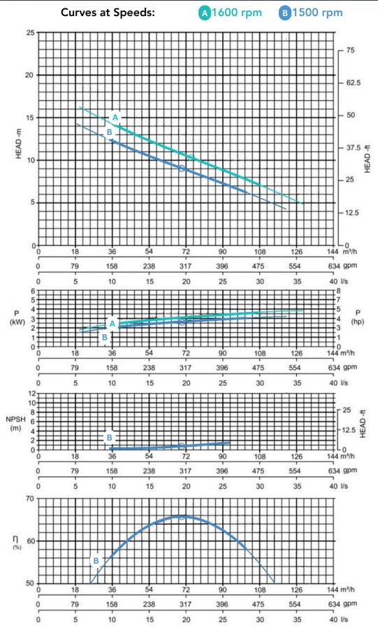
Note: Pump power P include mechanical seal friction and bearing frame losses, from a run in bearing frame. (Testing according ISO 9906:2012-38)
